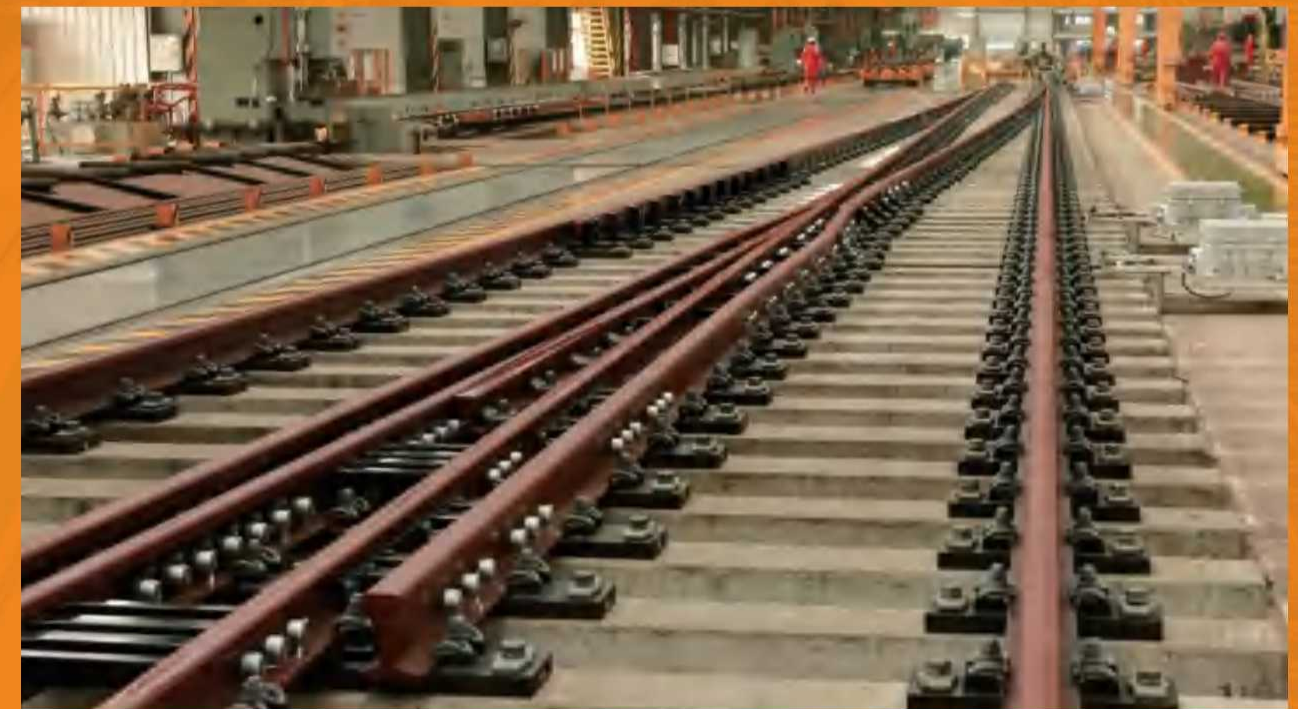
印尼雅万高铁350公里高速道岔 350km/h high-speed turnouts of JakartaBandung High-Speed Railway
