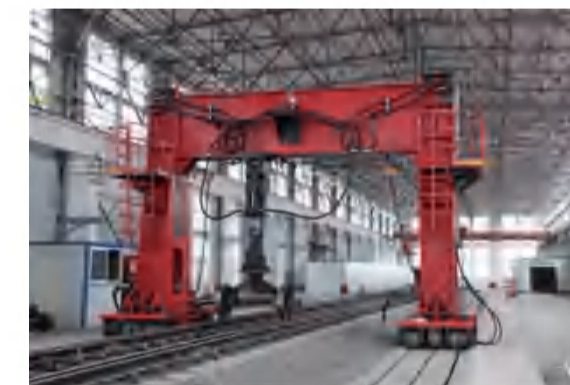
道岔足尺综合试验系统 Full scale comprehensive test system of turnouts
