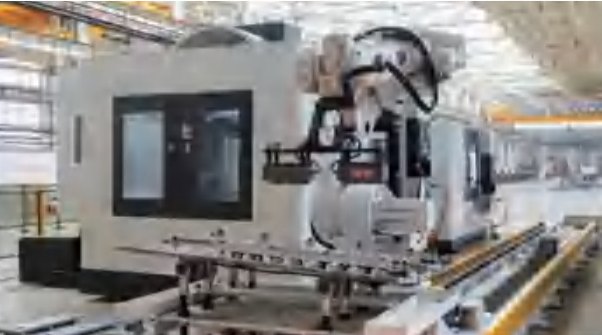
道岔垫板全自动数控加工集成单元 Fully automatic CNC machining integrated unit for switch base plate
