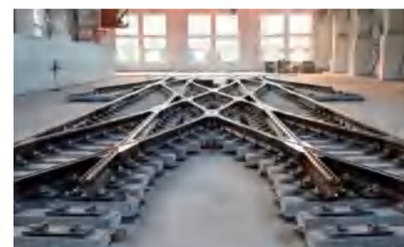
武汉现代有轨电车三开组合道岔 Modern tramway three-throw combination turnouts for Wuhan
