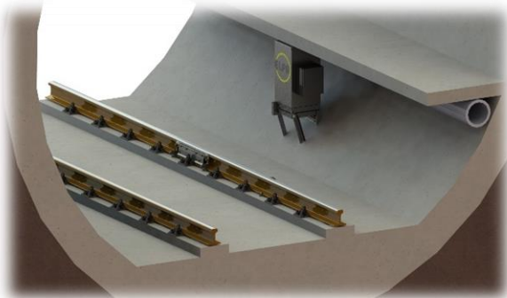
Main supply unit in tunnel under the pathway
